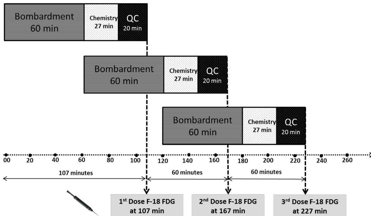
**Figure 2:** Workflow of cyclotron from bombardment, radiochemistry and quality control of final <sup>18</sup>F DG production for three successive runs of the cyclotron.
